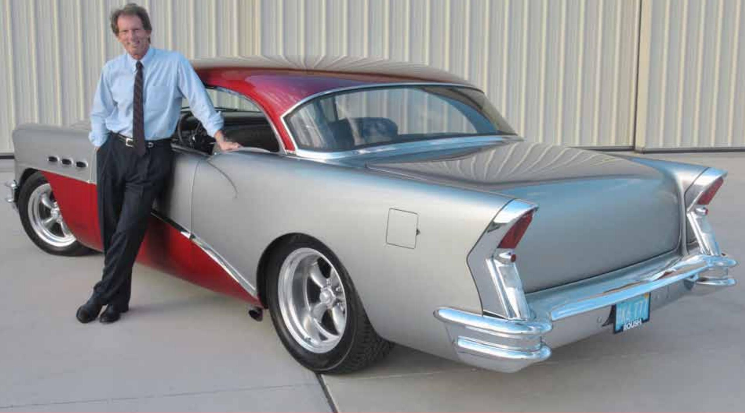
that roughly 30 percent of the chrome on the car has been eliminated. Few, however, will spot the subtleties like the original front bumper shape that has been thinned slightly with approximately one inch of depth
